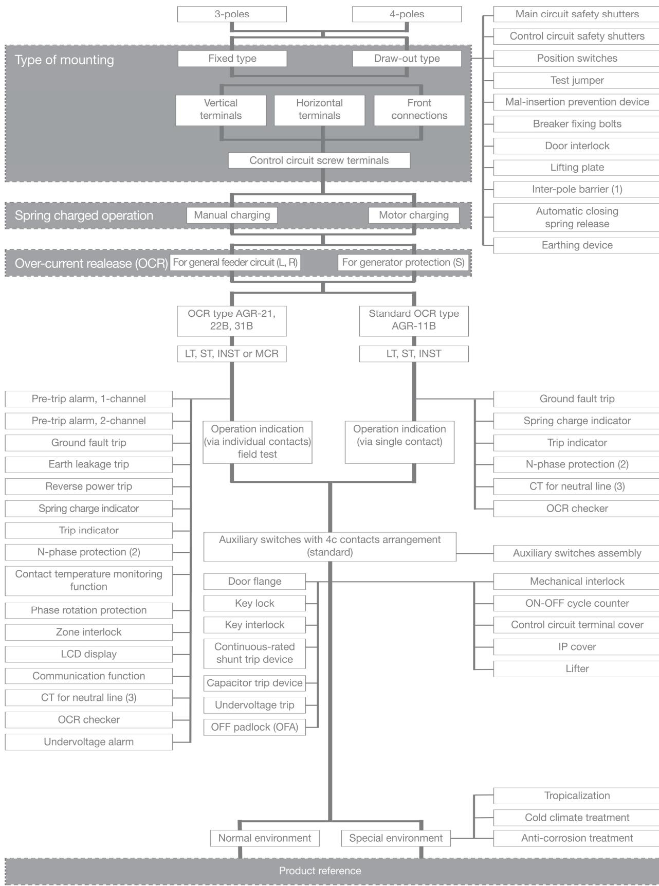
(1) : not applicable to ACBs equipped with front connections.
